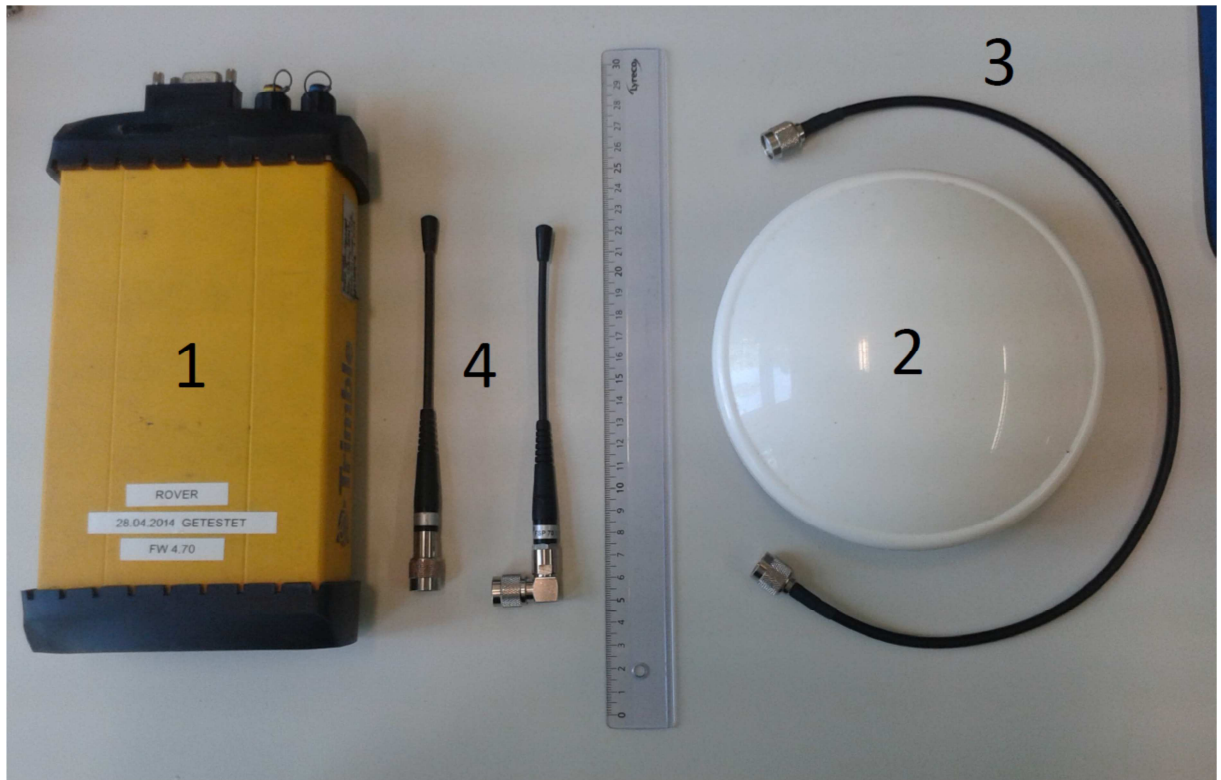
Picture 3 – GNSS system (Trimble AgGPS RTK Base 450): (1) receiver, (2) antenna Trimble AG25 GNSS with magnetic base, (3) cable for connecting the satellite antenna to the receiver and two options regarding the (4) radio antenna for RTK correction signal. No power supply is required due to built-in battery.
